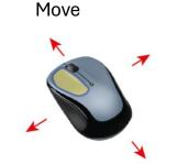
The left mouse button is held down to fly in viewing direction. Moving the mouse while holding down the left mouse button changes the flight direction, but not the altitude.
