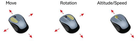
Moving the 3D section happens by pressing the left mouse button while moving the mouse simultaneously (click drag gesture). The process might be optionally repeated several times for the bridging of greater distances. The strength of the displacement is depending on the preset airspeed.
