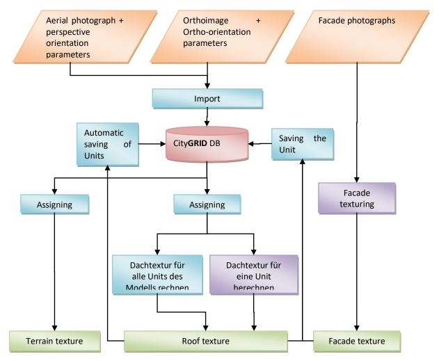
Roof and terrain are textured automatically, if a texture image together with its correct orientation parameters was imported into the data source and is assigned to the Model. The facade texture is assigned interactively or fully automatic from oriented images.
